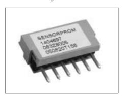
The factory settings matching the sensor are stored in the SENSORPROM® unit. Also customer specified settings are downloaded to the SENSORPROM® unit. Should the signal converter be replaced, the new converter will upload all previous settings and resume measurement without any need for reprogramming.
