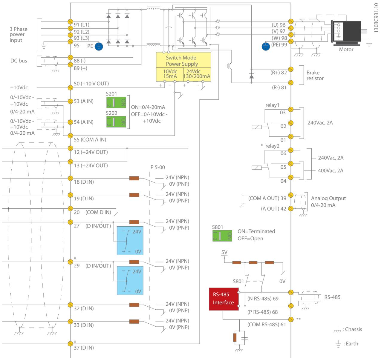
The diagram shows the terminals of the FC 301 and FC 302. Additional options will expand the number of terminals.
